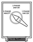
Figure 26. Voltage Selector Switch 480/277V
